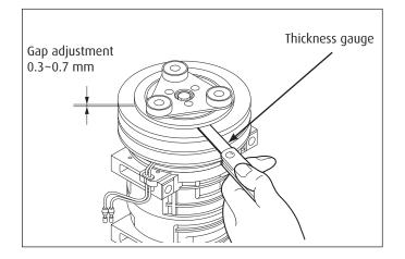
7. Check that the clutch clearance is as specified. If necessary adjust the clearance using shim(s).Adjusting shims are available in the following thickness:
