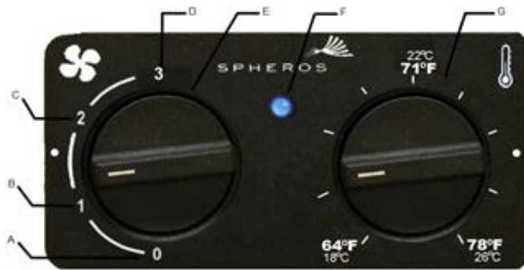
Fig. 2: Manual Control Panel
