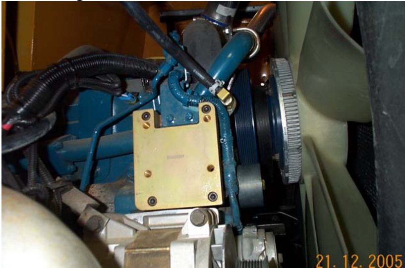
Install BMN60001 & Rotate Turbo intake tube away from Alternator.
