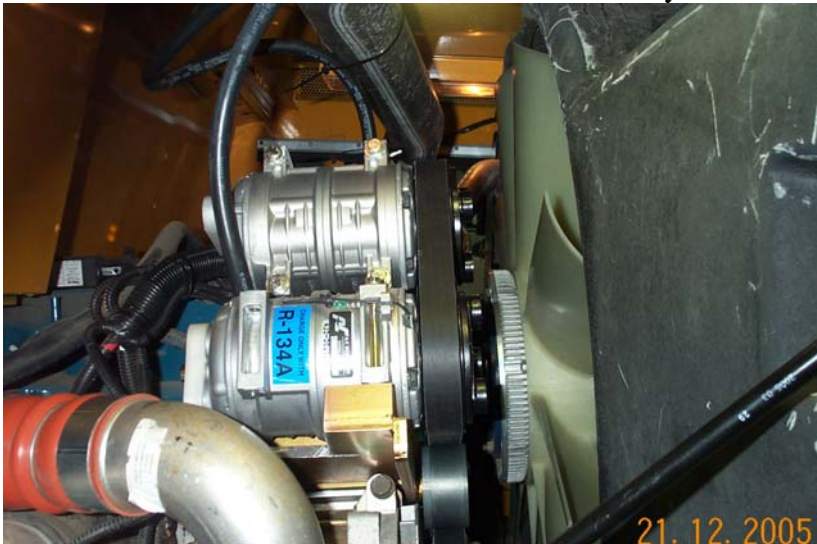
Mount Main Bracket, secure all hoses and tubes and check belt alignment.
