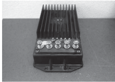
Motor Drive Controller
