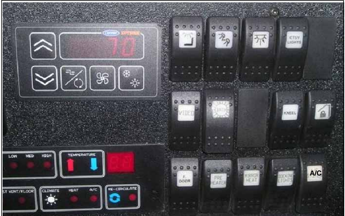
Figure 3-1 Bus Dash With A/C Switch & BT324 CSDD Controller
