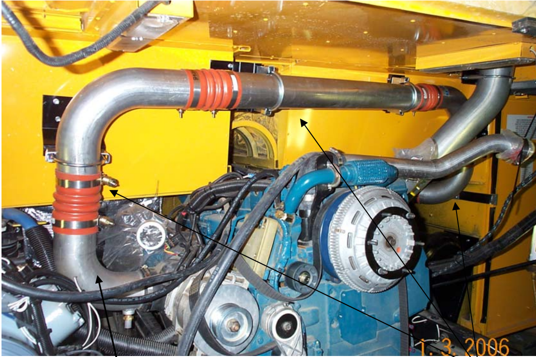
Air Filter and Air Intake stack is moved to curbside of bus. See Photos below
