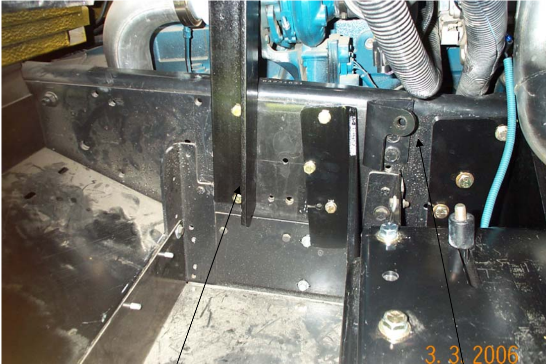
Install BMN80022 Rad Support Bracket and re-assign Rad Support Rod from OEM position to new position on BMN80023 at top of Rad Support Bracket.
