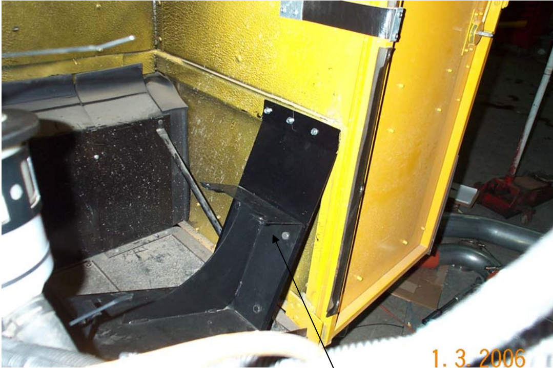
Navistar Air Filter brackets mounts on our BMN60007 bracket mounted on curbside.
