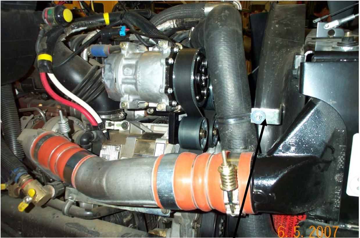
Rad hose is reversed and hose is supported from Rad shroud.
