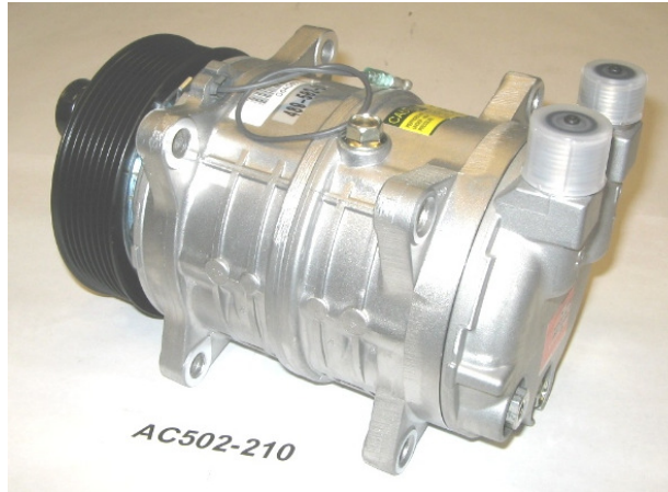
18-00093-05 Compressor, TM-16, (8) Grv., Poly-V, 12 VDC, Ear Mount, Vertical O-Ring, Monolithic Head, (was AC502-210)
