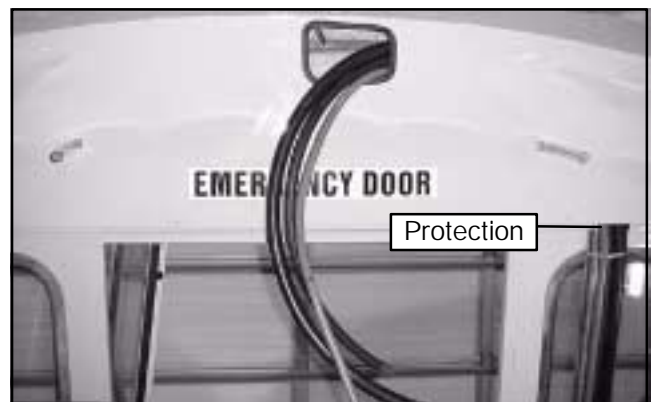
Figure 4-10 Hoses Routed Through Access
