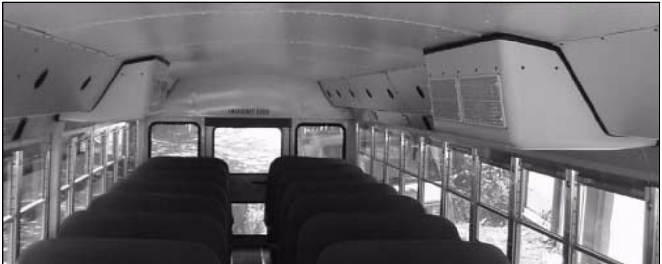
Figure 2-29 EM-9 Ducted Evaporator - Location - Completed Assembly
