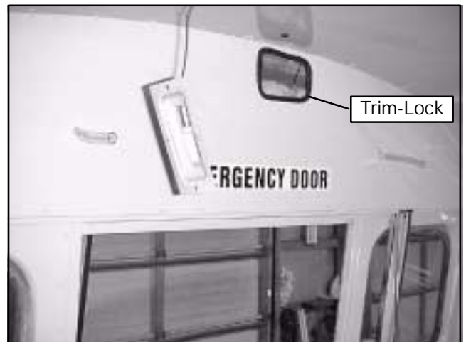
Figure 4-9 Access Hole With Trim-Lock
