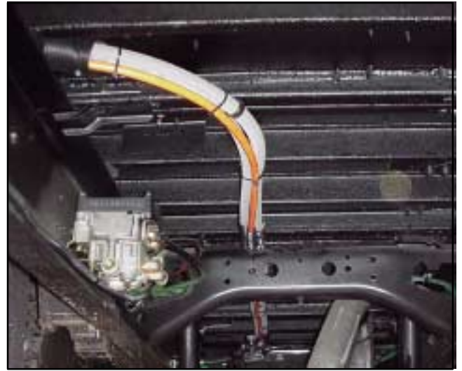
Figure 4-17 Hose Routing (Chassis)
