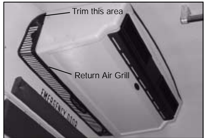
Figure 2-15 Return Air Grill
