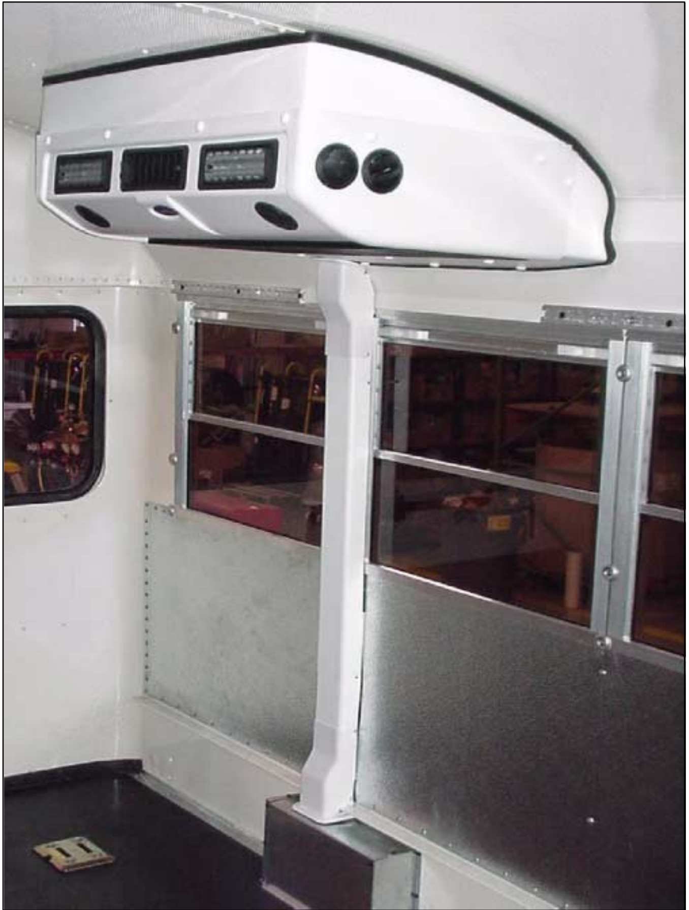
Figure 2-25 EM-2 (Gen V) Side-Mount - Free Blow, Installed (Complete)
