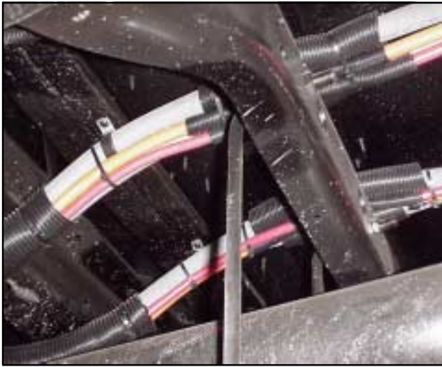
Figure 4-15 Hose Routing (Chassis)
