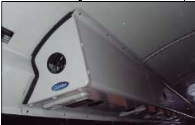
Figure 2-30 School Style Ducting-Passenger Side
