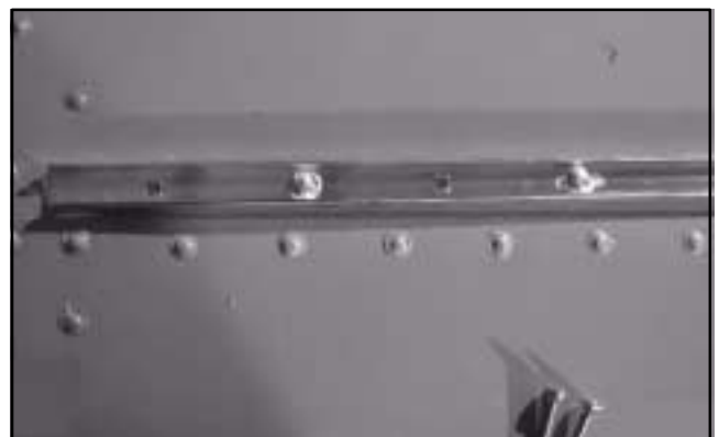
Figure 2-7 Carriage Bolt Sealing
