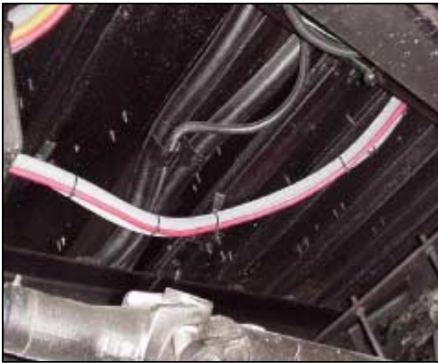
Figure 4-16 Hose Routing (Chassis)
