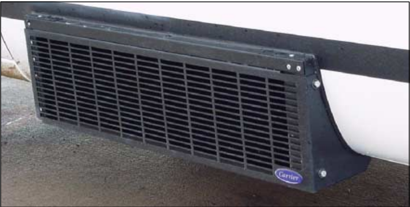
Figure 3-5 CM-2 Condenser Mounted on an Extended Roof Van (Custom)
